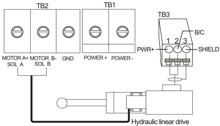
**How to connect the Accu-Steer FPS 12V/24V helm sensor**
