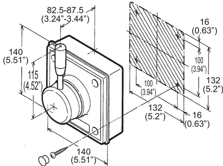
To mount the FAP-6221/6212 in a panel, the optional flush mount kit OP64-4 or OP64-5 is required.
