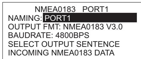
2. The cursor is selecting [NAMING: PORT1]. This menu item lets you change the name of the port. For example, equipment type, model number, etc. The name can have a maximum of 14 alphanumeric characters. If you don't need to change the name, go to step 3.
