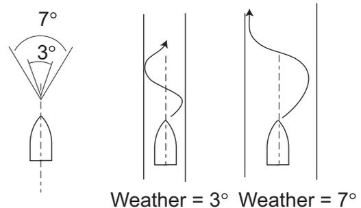
**[RUDDER GAIN]:** When the boat's heading deviates from the set course, the NAVpilot adjusts the rudder to correct it. The rudder angle (number of degrees) which is steered against every degree of course deviation is known as the rudder gain.
