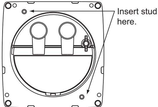
3. Set the unit to the mounting hole. Fasten the unit with the flat washers, spring washers and wing nuts (supplied).
