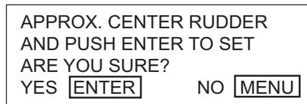
17. Turn the helm so rudder is centered then push the knob. The [RUDDER LIMIT SETUP] menu appears.
