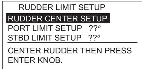
Set the rudder center position, then set the maximum rudder limits or “hard-over” points for the rudder system.
