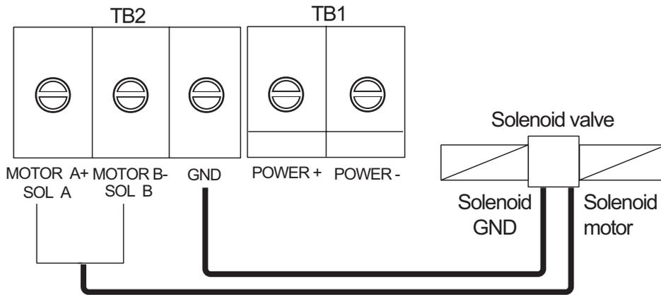
**How to connect a hydraulic linear drive**
