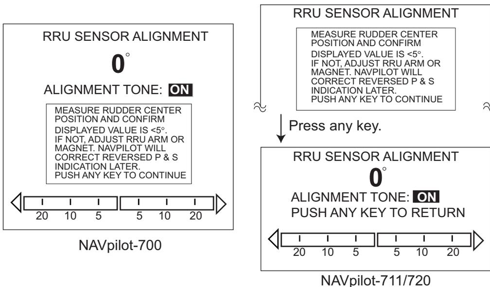
5. With the rudder physically centered, confirm that the displayed rudder angle indication is less than or equal to  $\pm 5^\circ$ . If not, you must adjust the rudder sensor body or magnet position (for Teleflex linear sensor AR4502) so that the indicator is within  $\pm 5^\circ$  before continuing.
