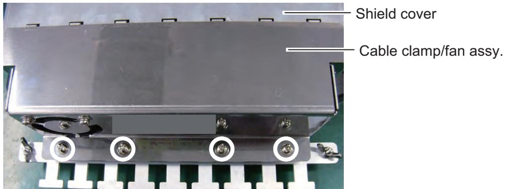
3. Separate the cable clamp/fan assy from the shield cover as shown in the figure below. Open the assembly carefully to prevent damage to the cable connected to the fan.
