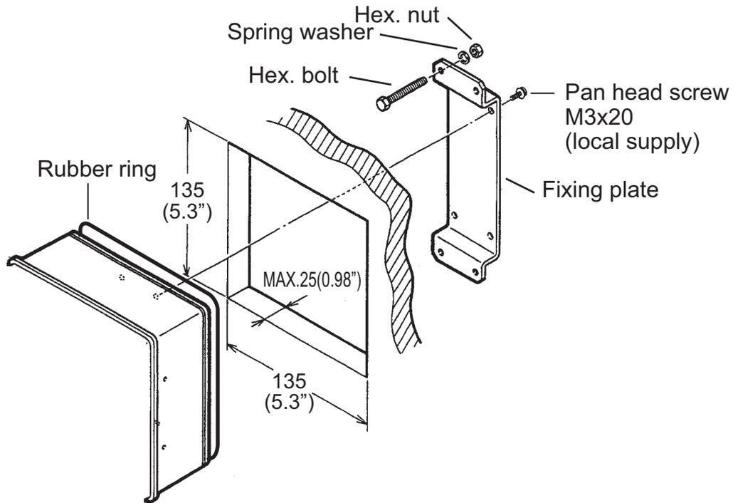
*How to flush mount the FAP-6221 with flush mount kit OP64-5*
