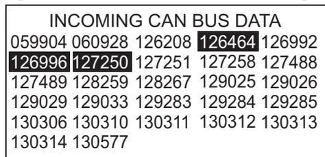
This display shows all the NMEA 2000 sentences that the NAVpilot is capable of receiving. The Parameter Group Number (PGN) the NAVpilot is currently receiving are highlighted.
