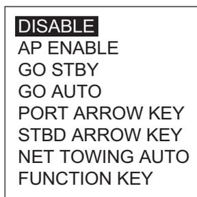
2. Rotate the knob to select the command or function for [IN PORT1]. This is the command or function assigned to the switch box connected to this port.
