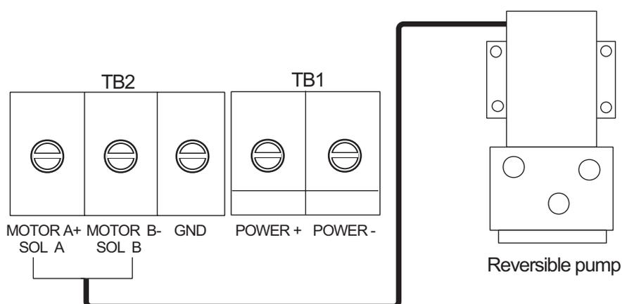
**How to connect a solenoid drive**
