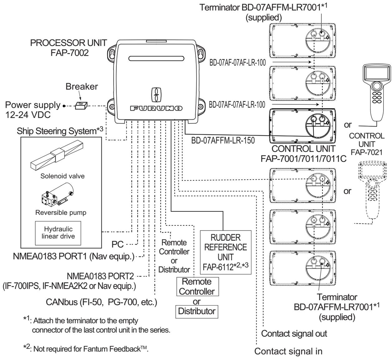
\*1: Attach the terminator to the empty connector of the last control unit in the series.
