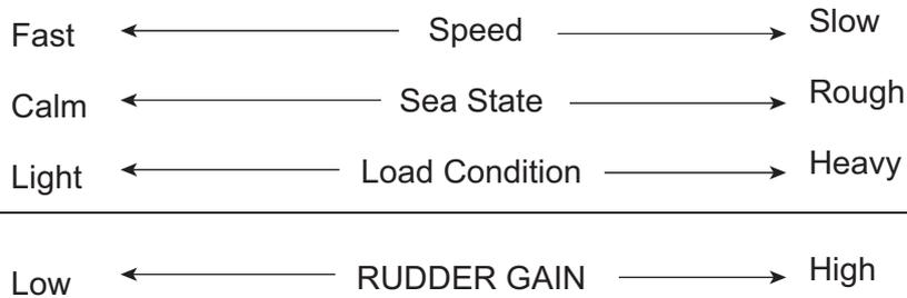
**[COUNT RUDDER]:** If the boat is heavily loaded, the heading could change excessively because of inertia. This phenomenon causes the vessel to “overshoot” the intended course. If this happens, the NAVpilot will steer the rudder to the opposite side and the heading will turn in opposite direction excessively again. In an extreme case the heading oscillates several times until it finally settles in the new course. An adjustment known as “counter rudder” prevents this kind of oscillation.
