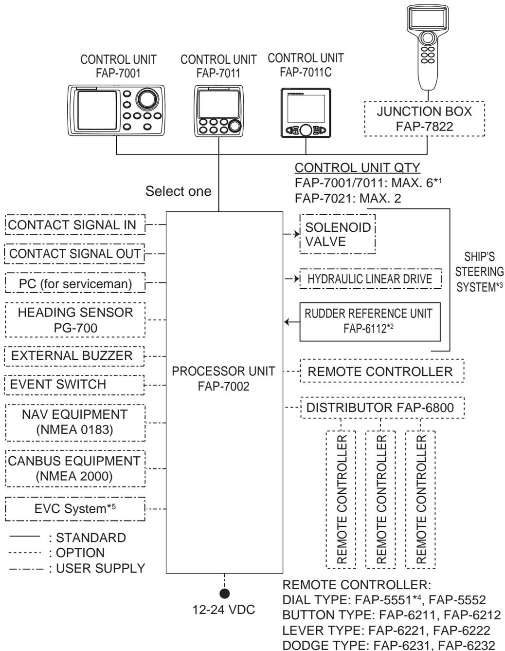
\*1: Any combination of control units is available. For FAP-7021, connect at the end of series.
