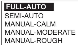
2. Rotate the knob to select the option which best matches current sea state then push the knob. For items other than [FULL-AUTO], go to step 4.
