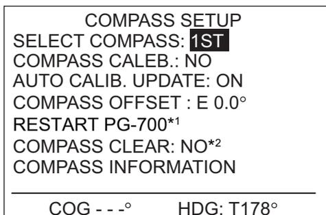
\*1 Appears with connection of PG-700. Restarts PG-700. Turn the steering mode to the STBY mode to restart PG-700.
